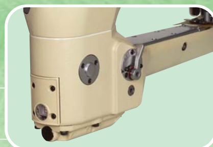
右邊搖桿可調後牙差動及大、小針距。 The right side lever can adjust the rear differential feeding and stitch length.
