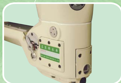
左邊搖桿可調前牙差動 The left side lever can adjust the front differential feeding
