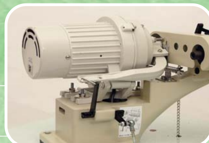
改變傳動方向之轉換接頭 The connector of changing the driving direction
