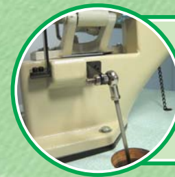
專利---機座型離合器馬達連桿設計。 Patented---Innovative design of pitman rod for the clutch motor sits on machine's body.
